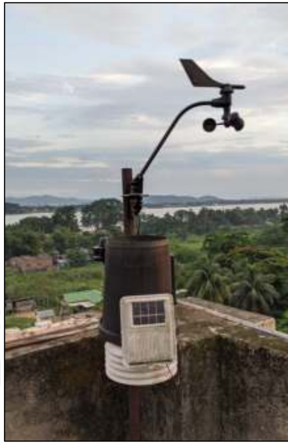
Fig. 3.4 Wireless weather station (Vantage pro2, USA) installed at the Air Pollution Laboratory, IIT Guwahati rooftop.
