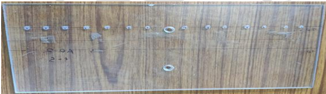
Figure 3.12: Flat-plate wing with inverted dimples at 0.25c location
