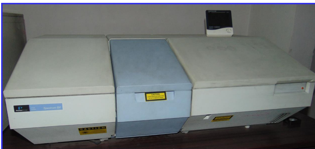
Figure 2.11: Photograph of the FTIR spectrometer (Perkin Elmer, Spectrum BX).
