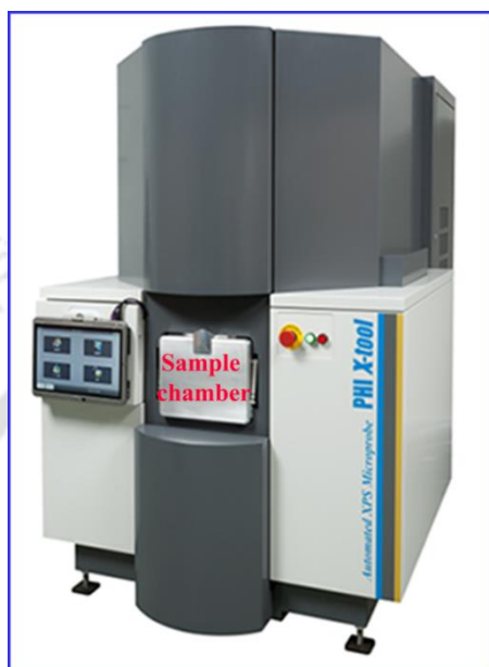
Figure 2.13: Photograph of the X-ray photoelectron spectrometer (ULVAC-PHI, Inc.).
