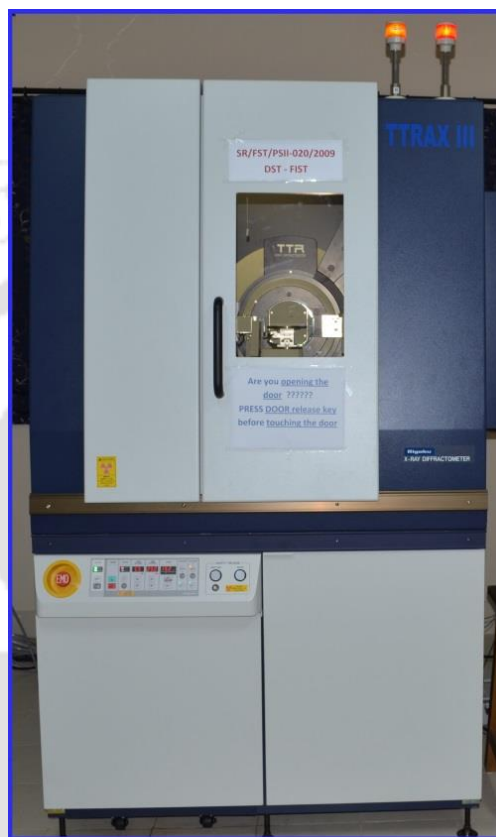
Figure 2.14: A photograph of the X-ray diffractometer (Rigaku RINT 2500, TTRAX III).
