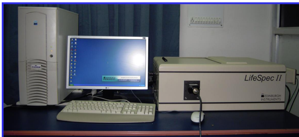
Figure 2.10: Photograph of the TRPL spectrometer (LifeSpec II, Edinburgh Inst., UK).
