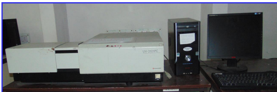
Figure 2.7: Photograph of the UV-Vis absorption spectrometer (Shimadzu, UV3101PC).
