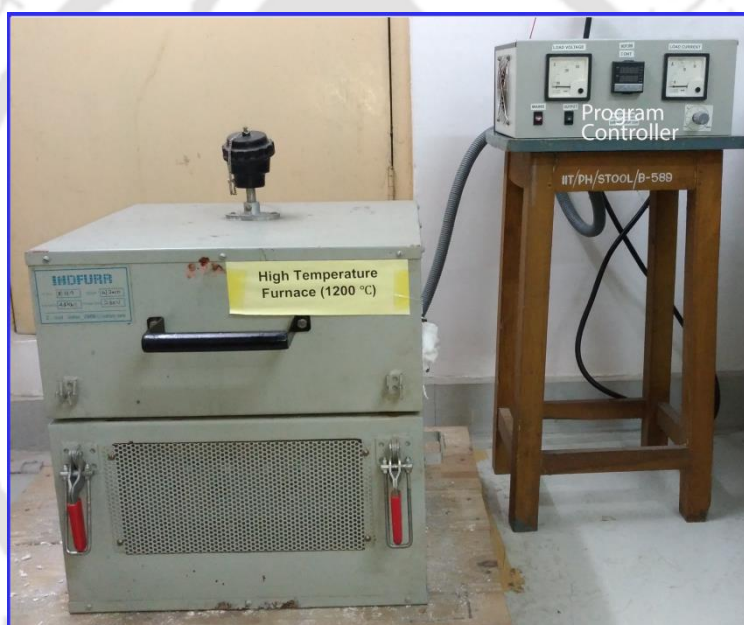
Figure 2.2: Photograph of high temperature furnace (Indfurr, India) and temperature controller unit.
