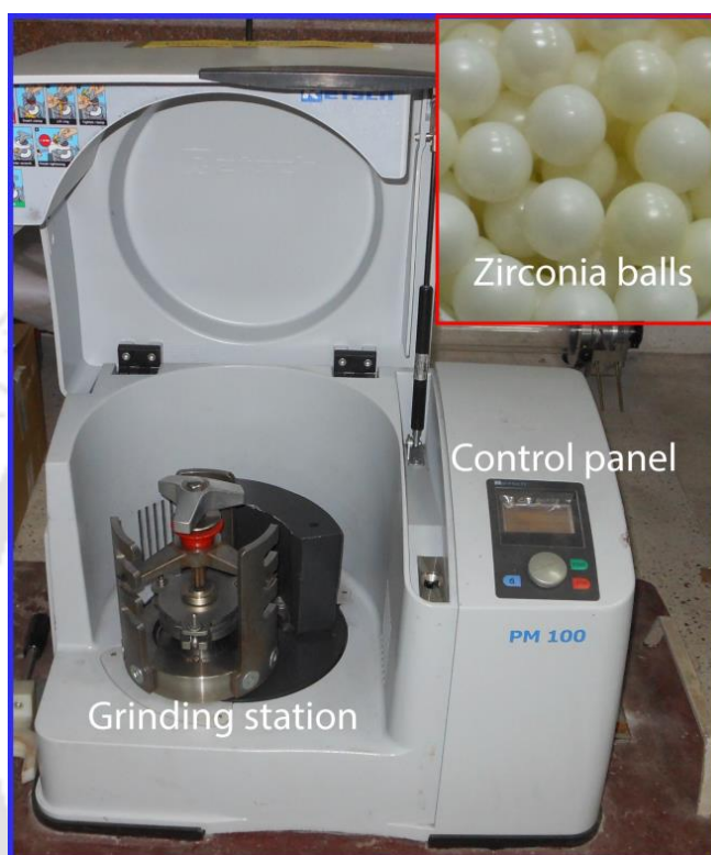
Figure 2.3: Photographs of the planetary ball-mill machine (Retsch, PM 100), grinding station and zirconia balls.
