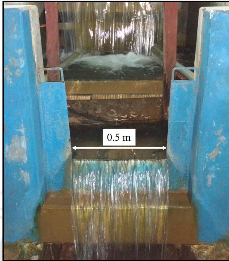
Figure 2.6 Discharge measurement at rectangular notch.
