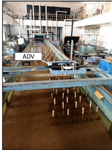
Figure 2.9 Snapshot of Acoustic Doppler Velocimeter (ADV) capturing velocity measurement.
