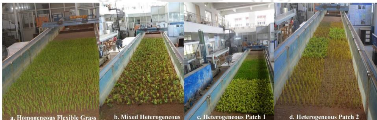
Figure 1.9 Snapshots of different homogeneous and heterogeneous vegetated zone layout with uniform vegetation height (Courtesy: Chembolu et al. 2019)
