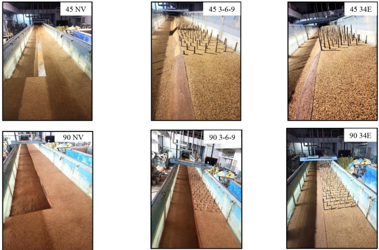
Figure 2.17 Snapshots of Experimental cases for Set-up 1/ 45^{\circ} bank slope and Set-up 2/ 90^{\circ} bank slope compound channel
