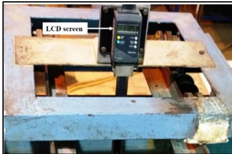
Figure 2.7 Digital point gauge.
