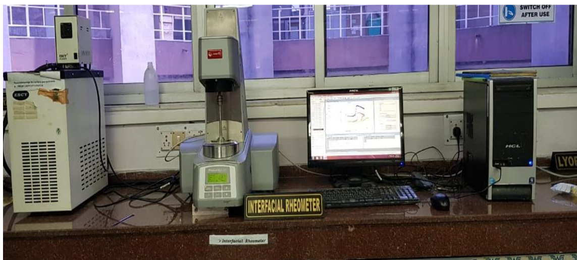
Figure 3.5 Pictorial representation of Anton Paar MCR 301 rheometer
