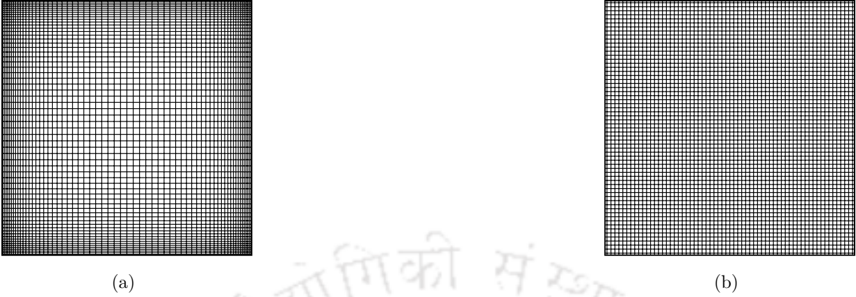
Fig. 3.2: A 65 \times 65 grid in (a) physical plane and (b) computational plane.
