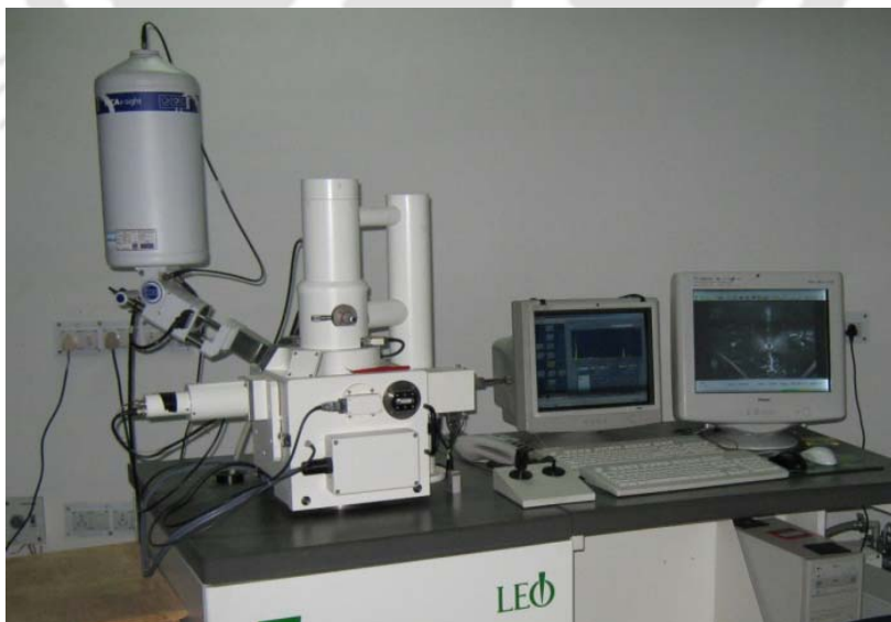
Figure 2-2: Photograph of the Scanning electron microscope used (LEO 1430 VP).
