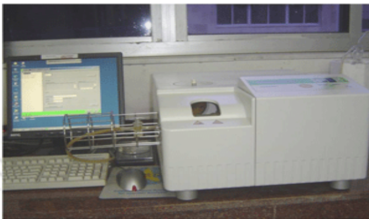
Figure 2-10: Image of the TGA /DTA instrument used (Metler–Teledo TGA 1100).
