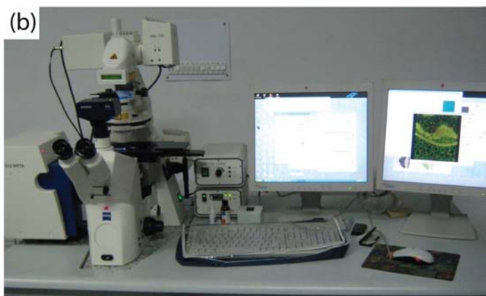
Figure 2-6: Photograph of CLSM used (Model. Zeiss LSM 510 Meta)
