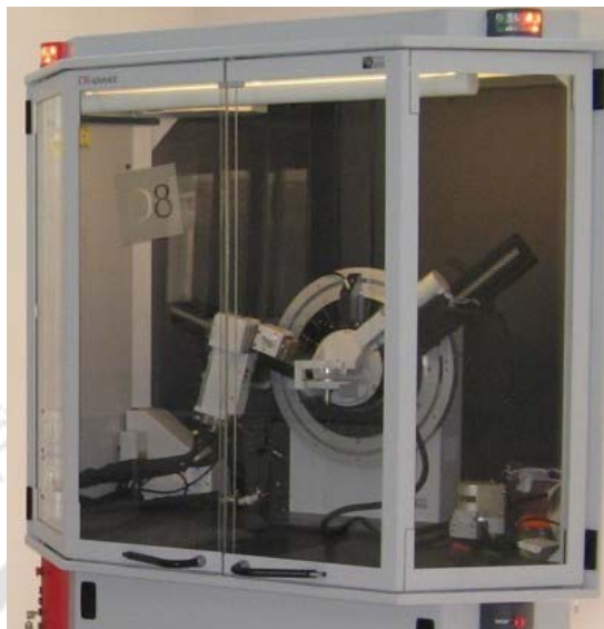
Figure 2-9: Photograph of the powder X-ray diffractometer used (Model: Bruker D8-Advanced tools).
