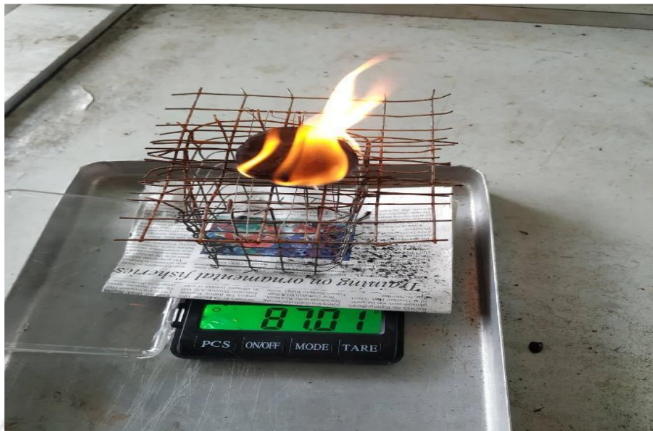
Figure 4.7: Photograph of the setup of open burning combustion test of briquette sample.
