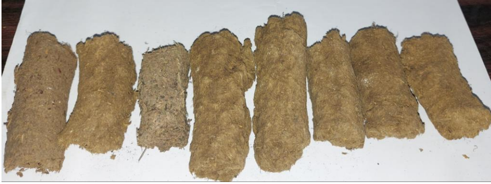
Figure 4.1: Photograph of briquette made from grass, dry leaves and straw
