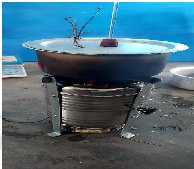
Figure 4.6: Photograph of the Setup for the water boiling test
