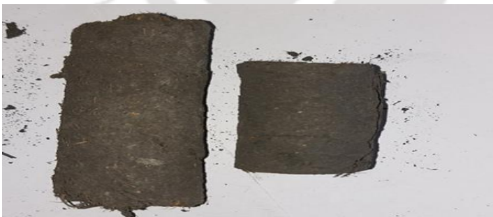
Figure 4.14: Photograph of briquette from carbonised rice straw using screw press machine
