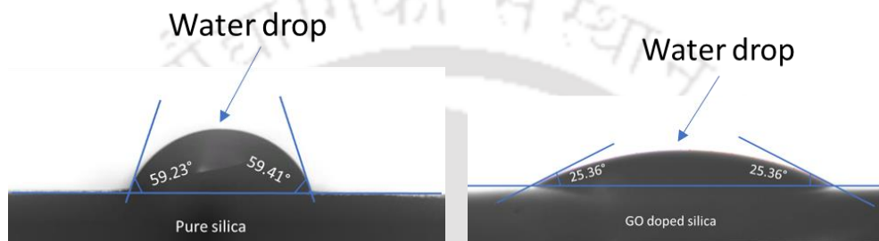
Fig 2.6 : Contact angle measurement of water droplet on (a) pure sol-gel silica substrate (b) GO diffused nanostructured sol-gel silica substrate.
