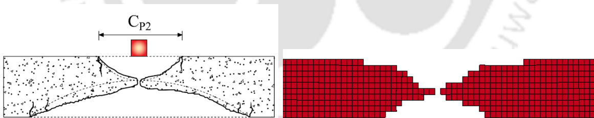
Figure 2.6 Panel at initiation of Perforation (P2)
