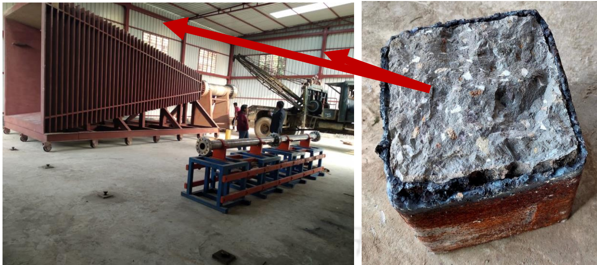
Figure 10.17 Strong floor with High compressive strength of concrete in Blast and Impact Resistant Prototype Building at IIT Guwahati having present day Compressive Strength of 134.5 MPa
