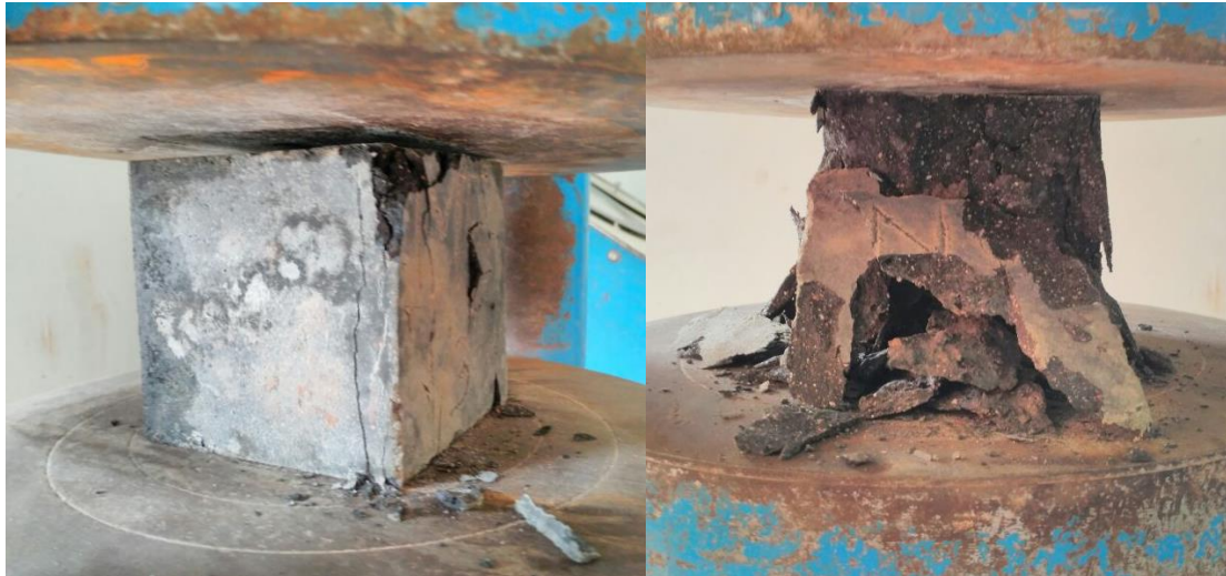
Figure 9.18 Compressive Strength Testing of Cubes
