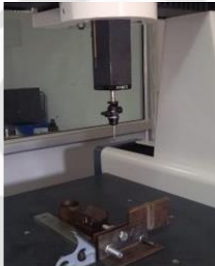
Figure 4.9 Surface deformation measurement on CMM
