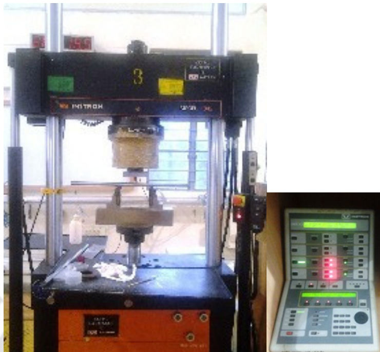
Figure 6.6 Intron machine and its display console
