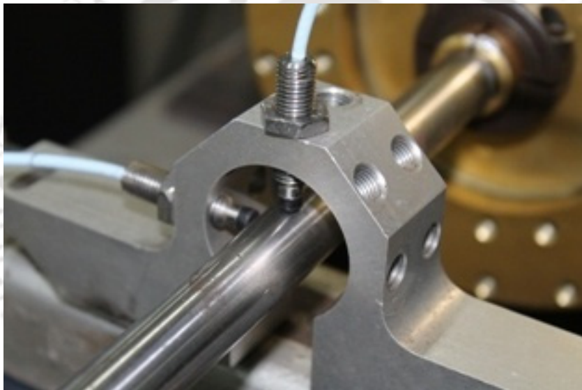
Figure 6.12 Eddy Current proximity probes for displacement measurement in two orthogonal transverse directions
