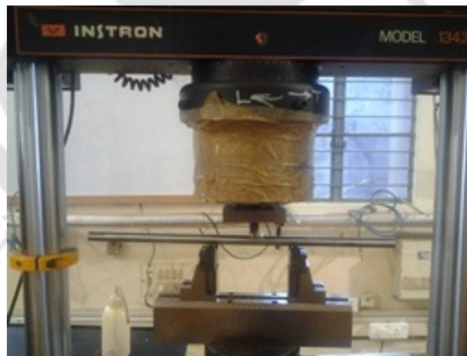
Figure 6.7 Test shaft in the three-point bending fixture
