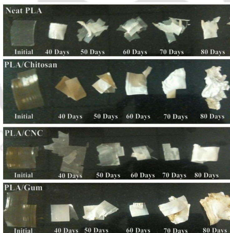
Figure 4. 9: Samples were randomly taken out and weight at different times of composting duration. Samples are small pieces and cameras were zoomed before taking the pictures for better visibility.
