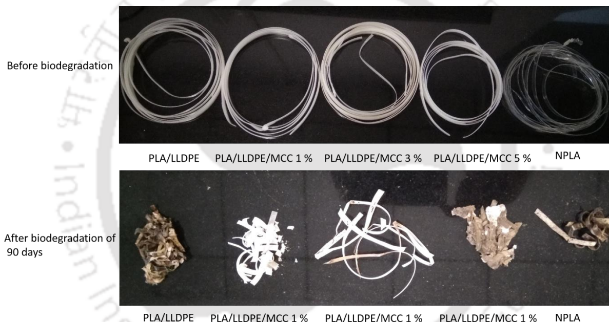
Figure 5. 1: Laboratory composting setup used for biodegradation study and the samples that were tested under the system.
