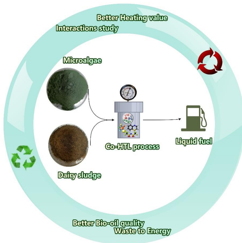
Figure 1.6. Co-Hydrothermal liquefaction of algal biomass with dairy sludge.
