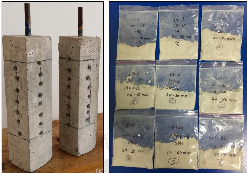
Fig. 3.19 Drilled prismatic specimens and sieved concrete powder samples
