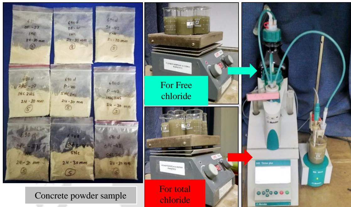
Fig. 3.15 Photograph during measurement of chloride concentration of SCC mixes
