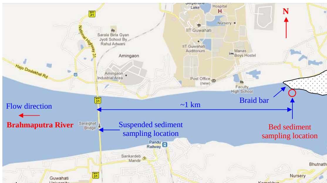
Figure 3.3: Bed sediment sampling location (Not to scale) (Source: www.google.com, as on 28-08-2011)
