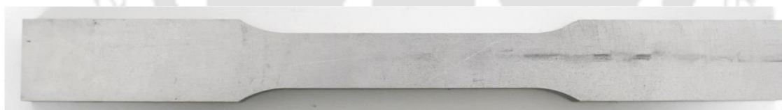
Fig. 4.15 Dog-bone-shaped tensile specimen fabricated using Al 7075-T6 alloy.
