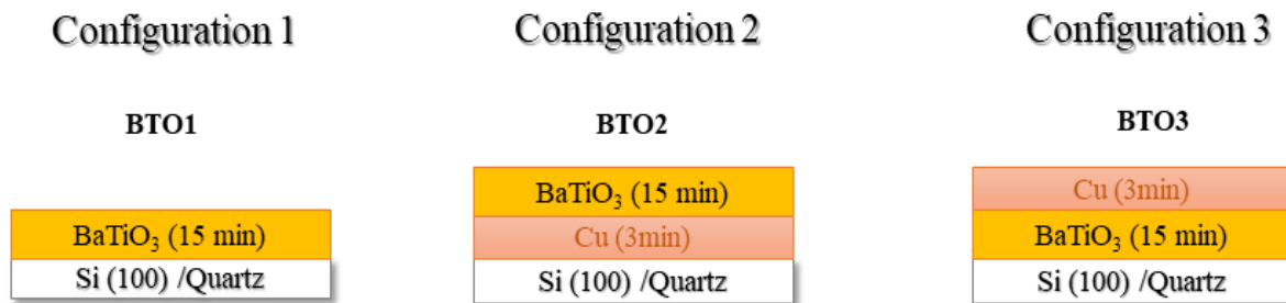
Figure 2-6 Cu infused BTO thin film configurations.
