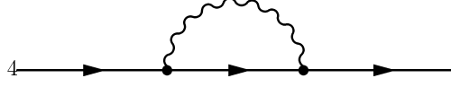
Figure 2.1: Self-energy correction. The self-energy \Sigma(\mathbf{k}, \omega) corresponds to the loop. Propagators are indicated by arrowed lines and correlation by a wiggly line.
