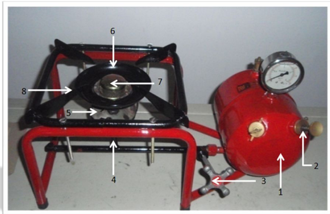
1: Fuel tank, 2: Hand operated plunger pump, 3: Fuel regulator, 4: Rising tube, 5: Spirit cup, 6: Heat shield, 7: Vapour burner with flame holder, 8: Pot holder.
