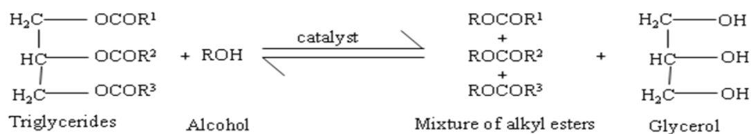
Fig. 2.5. Transesterification reaction of oil , where, R1, R2 and R3 represent the different fatty acid derivatives (long unbranched aliphatic tail (chain), which are either saturated or unsaturated)
