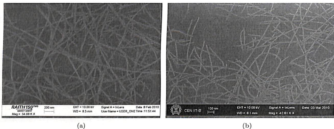
Figure 4.4: SEM images of SWCNT thin-film deposited on the functionalized surface by dip-coat method. (a) SWCNTs on Si/SiO 2 surface. (b) SWCNTs on Si/HfO x surface.
