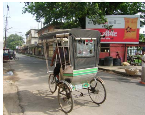
Fig. 7.44 Three quarter rear view of Dipbahan imitated at Guwahati in Assam with similar hood structure using a normal traditional rickshaw
