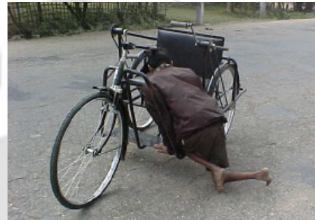
Fig 3. 8 Access to a tricycle is difficult due to constraint space & design
