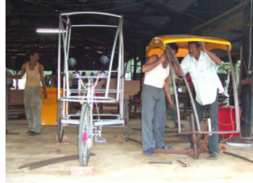
Fig. 5.38 Assembly of body from sub frames
