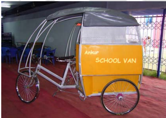
Fig. 7.23 Dipbahan Ankur school van has its length, breadth (of body) and height increased by 200 mm, 200 mm, 150 mm respectively compared to length, breadth and height of Dipbahan+
