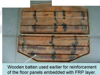
Fig. 4.7 Floor panels (shown above) and passengers' seat (not shown here) fabricated in FRP for Dipbahan + required reinforcement. Wooden battens were used prior to FRP battens using FRP wastes was available
