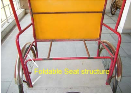
Fig. 5.23 Foldable seat structure
