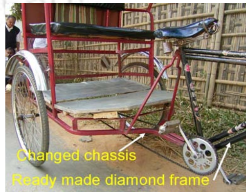
Fig. 5.31. Chassis modified by CRD
