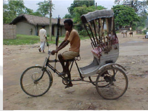
Fig. 6.2 Rickshaw in Guwahati, Assam with higher seat inclination to the front
