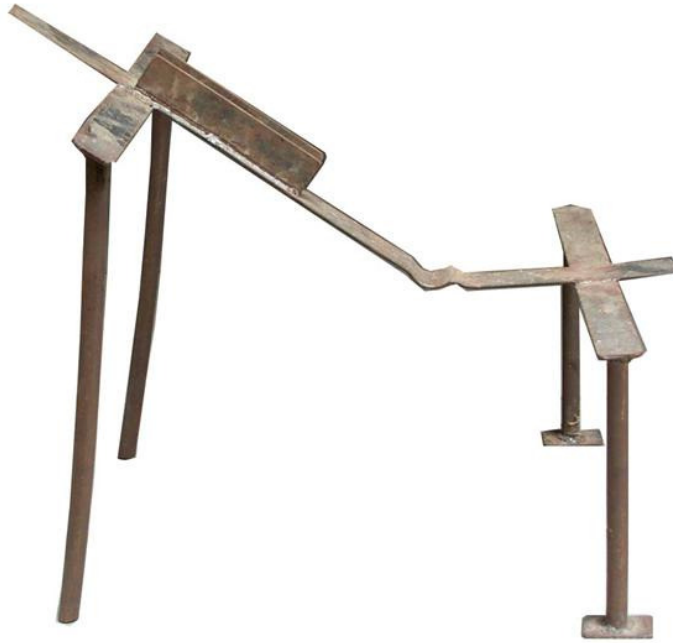
Jig_6 for assembly and joining of mainframe with body bottom socket
