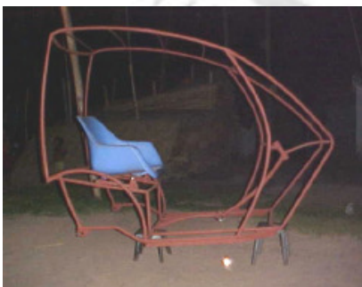
Fig. 3.30 Prototyped Body shell of the Trike Side view
