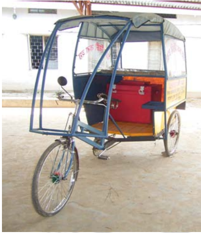
Fig. 7.26 Front three quarter view of the vending cart: it has the same dimensions as that of Dipbahan Ankur, the school van based on Dipbahan + including the side frames
