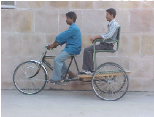
Fig. 5.1 Obtaining data using the traditional rickshaw platform; side view of layout with reduced leg space
