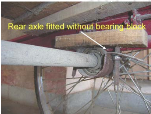
Fig. 5.32 Rear axle without bearing block
