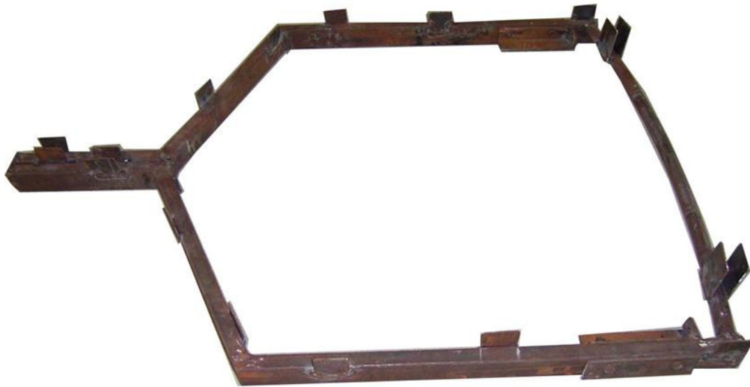
Jig_7 for assembly and joining of chassis elements
