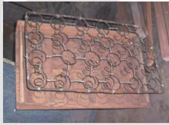
Fig. 2.35 Spring fitted passenger seat
