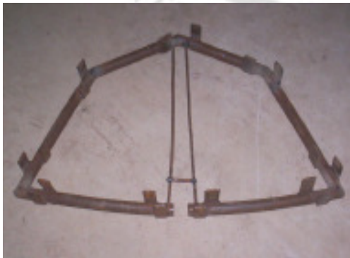
Fig. 7.8 Jig for the front end which is fitted to the main frame of the tricycle
