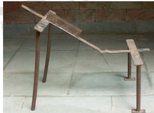
Fig. 7.9 Jig for joining the mainframe and chassis of the tricycle
