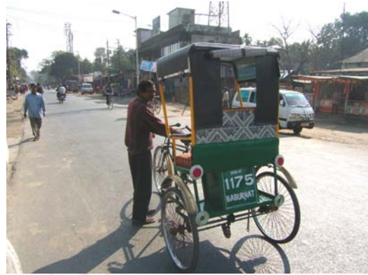
Fig. 7.34 Three quarter rear view of Dipbahan imitated at Coch Behar in North Bengal with similar rear end, seat and partial hood structure
