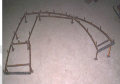
Fig. 7.5 Jig for the left side frame for body shell which is fitted on the main frame and chassis of the tricycle
