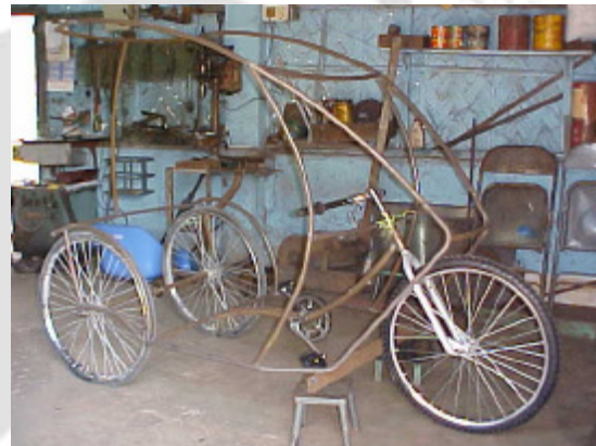
Fig. 3.29 Prototyping of the Trike in progress
