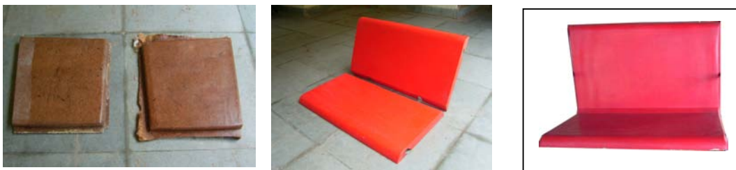
Fig. 5.39 Jute based Bio-composite Fig. 5.40 Seat in two piece Fig.5.41 Integrated single seat
