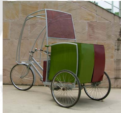
Fig. 7.22 Rear 3 quarter view of Pariskar, it has identical wheel base and track as that of Dipbahan+
