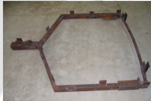
Fig. 7.7 Jig for the chassis which is fitted to the mainframe of the tricycle
