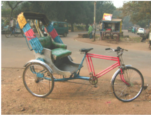
Fig. 6.1 Rickshaw at Kharagpur, West Bengal with less seat inclination to the front
