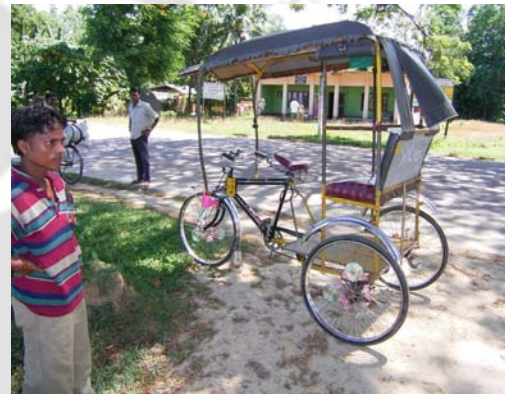
Fig. 7.42 Three quarter rear view of Dipbahan imitated at Bokakhat in eastern Assam with similar rear end, seat and hood structure
