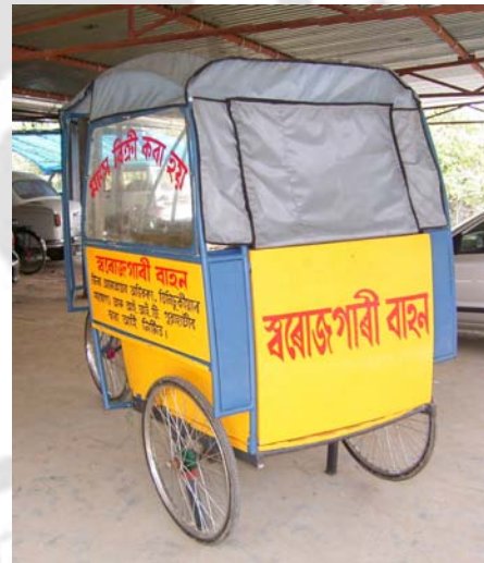
Fig. 7.28 Rear three quarter view of the vending cart with foldable screen cover and advertisement space
