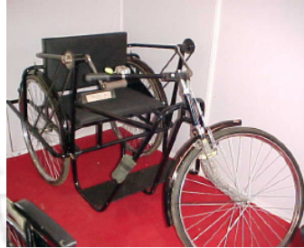
Fig. 3.2 Rear wheel driven with sprocket and chain
