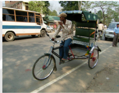
Fig. 7.30 Dipbahan imitated at Bokakhat in eastern Assam with similar rear end, seat and partial hood structure
