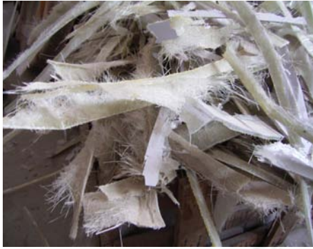
Fig. 4.3 FRP wastes generated from components as side trimmings
