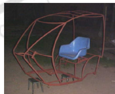
Fig. 3.31 Prototyped Body shell of the Trike 3 quarter front view
