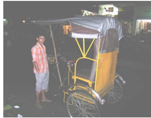
Fig. 7.40 Three quarter rear view of Dipbahan imitated at Tinsukia in eastern Assam with similar rear end, seat and hood structure but bus type seat
