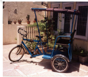
Fig. 2.41 Eco-Trike passenger rickshaw with 18-gears
