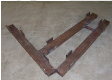
Fig. 7.6 Jig for the main frame which is fitted to the chassis of the tricycle
