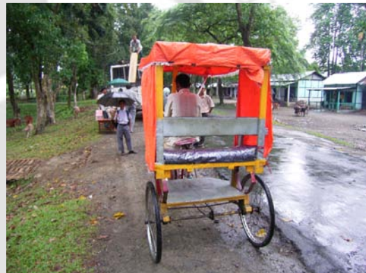
Fig. 7.36 Three quarter rear view of Dipbahan imitated in wood at Sadiya in Eastern Assam with similar rear end, seat and hood structure
