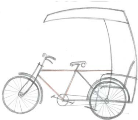
Fig. 3.44 Concept 5 -rickshaw based on a bicycle and a side car in mild steel structure with extended canopy
