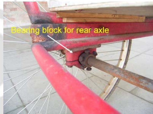
Fig. 5.33 Bearing block as per specification
