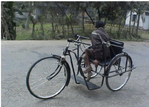
Fig 3. 11 Rear viewing is difficult without rear view mirror
