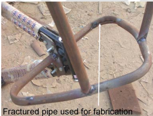
Fig. 5.34 Pipe fractured during bending
