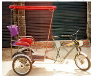
Fig. 2.40 Eco-Trike passenger rickshaw with shocker fork
