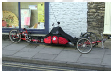
Fig. 1.25 Trice X2R back-to-back - A Special purpose recumbent tricycle
