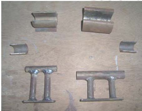
Fig. 7.12 Press tools to make U shape brackets
