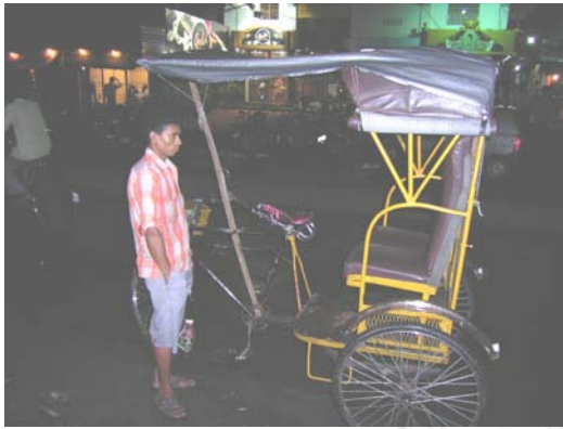
Fig. 7.39 Three quarter front view of Dipbahan imitated at Tinsukia in eastern Assam with similar rear end, seat and hood structure but bus type seat
