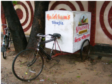
Fig. 2.19 Closed box type delivery van Delta configuration
