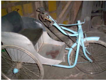
Fig. 3.1 Front wheel driven driven with sprocket and chain
