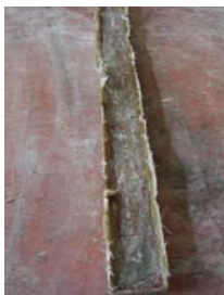
Fig. 4.3 FRP wastes generated from components as side trimmings
