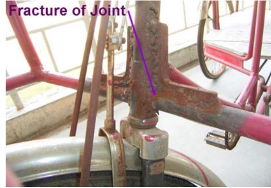
Fig. 5.24 Point of fracture
