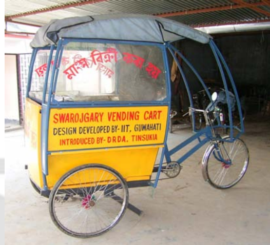
Fig. 7.27 Side view of the vending cart, it has its length, breadth (of body) and height increased by 200 mm, 200 mm, 150 mm respectively compared to length, breadth and height of Diobahan +
