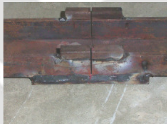
Fig. 7.2 Jig for cutting tubes at right angle
