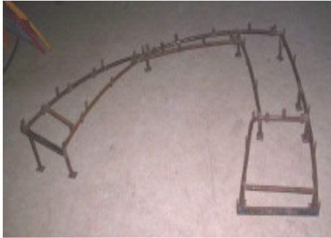
Fig. 7.4 Jig for the right side frame for body shell which is fitted on the main frame and chassis of the tricycle
