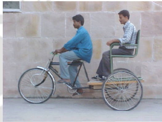
Fig. 5.2 Obtaining data using the traditional rickshaw platform; side view of layout with enhanced leg space
