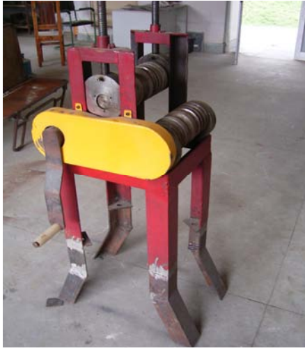
Fig. 4.1 Three quarter rear view of roller type pipe bending machine fabricated specially for the project purpose in the workshop of Department of Design
