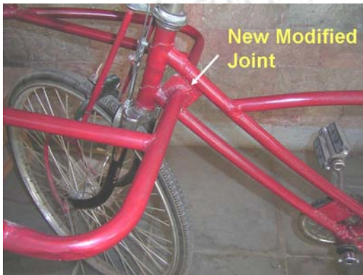
Fig. 5.25 Modified front end joint
