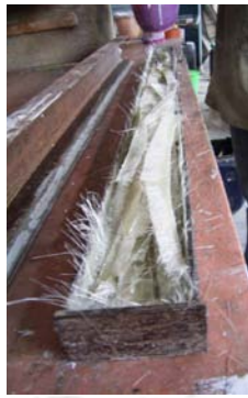
Fig. 4.4 FRP wastes placed inside mould
