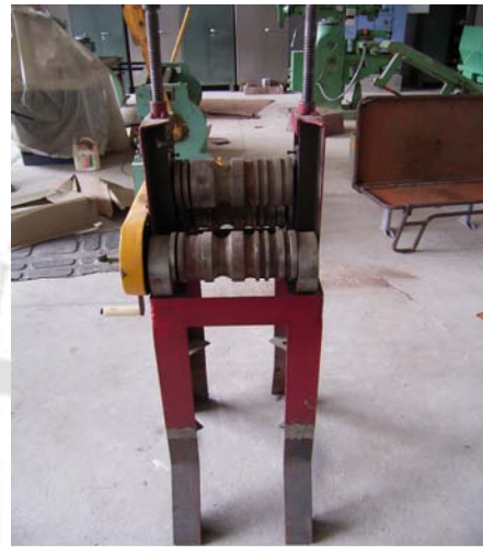
Fig. 4.2 Rear view of roller type pipe bending machine fabricated specially for the project purpose in the workshop of Department of Design
