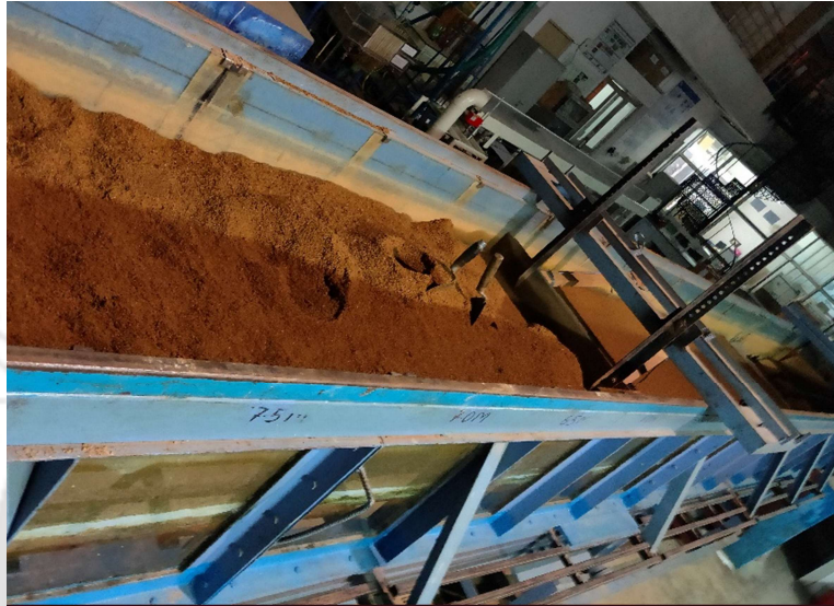
Figure 2.3: Channel Bed Preparation
