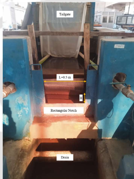
Figure 2.4: Rectangular Notch to Measure Flow Rate
