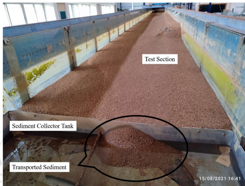
Figure 2.8: Sediment Collector Tank
