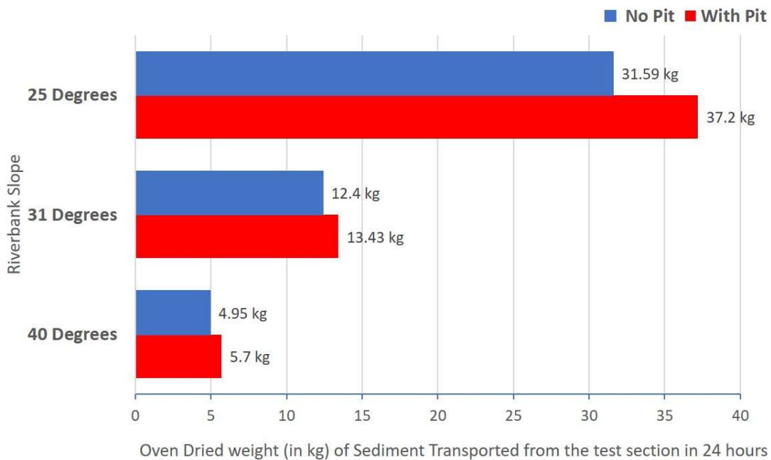
Figure 3.13: Sediment Transported through the Test Section in 24 Hours of the Experimental Run
