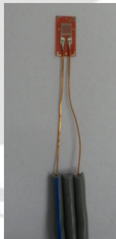
Figure 6.16 A typical 1 mm gage length, pre-wired TML strain gage
