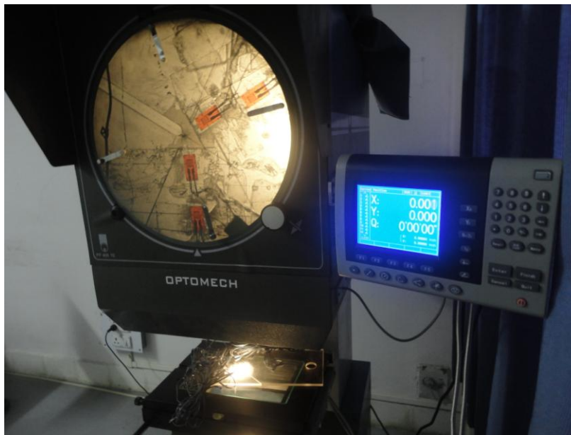
Figure 6.17 Profile projector for verification of orientation and location of a strain gage
