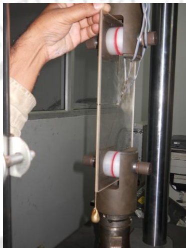
Figure 6.20 Checking of alignment of a specimen using plumb
