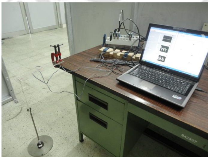
Figure 6.5 Cantilever beam testing setup
