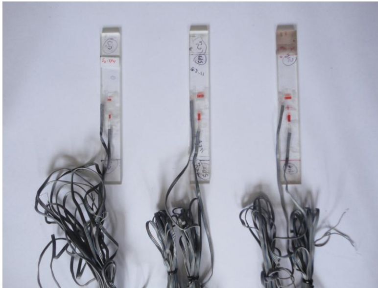
Figure 6.4 Rectangular specimens pasted with strain gages
