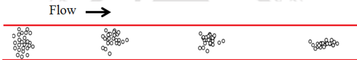
Figure 1.4. Schematic of shear induce migration phenomena.
