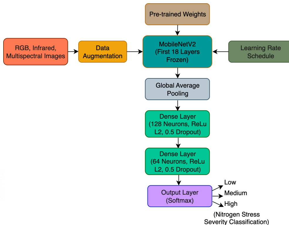
Figure 5.3: Spatial Deep Learning Framework for Nitrogen Stress Severity Classification
