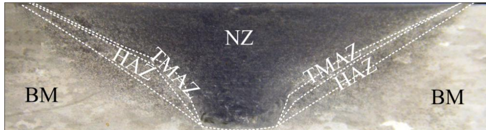
Fig. 3.10 Different metallographic zones in friction stir welded sample
