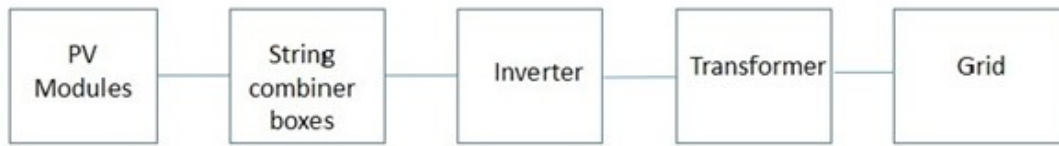
Figure 3.1: Simplified schematic diagram of a grid-connected PV system
