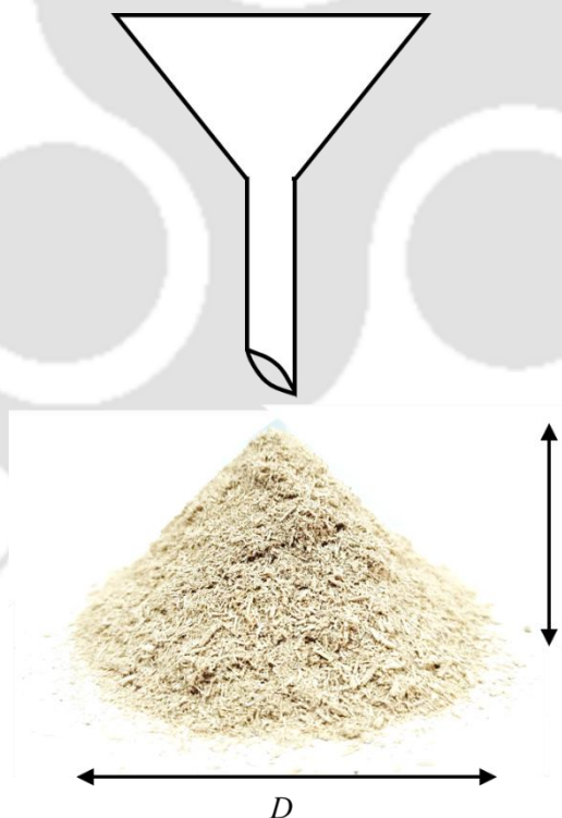
Figure 4.1.4 Schematic diagram for calculating angle of repose.
