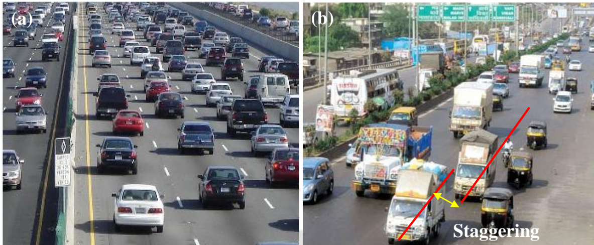
Fig 1.1 Traffic stream in (a) developed countries and (b) developing countries. Source- (a): I-80 Eastshore freeway in Berkeley, USA. ( https://en.wikipedia.org/wiki/Interstate_80_in_California ); and (b) Western Express Highway in Mumbai, India. ( images.mid-day.com/2012/nov/Kalanager.jpg ).
