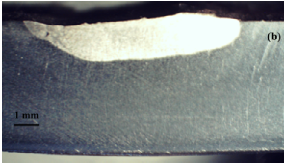
Figure 4.38: GTA weld macrographs using \text{Al}_2\text{O}_3 activating flux corresponding to (a) data set 1 and (b) data set 2 given in Table 4.8.
