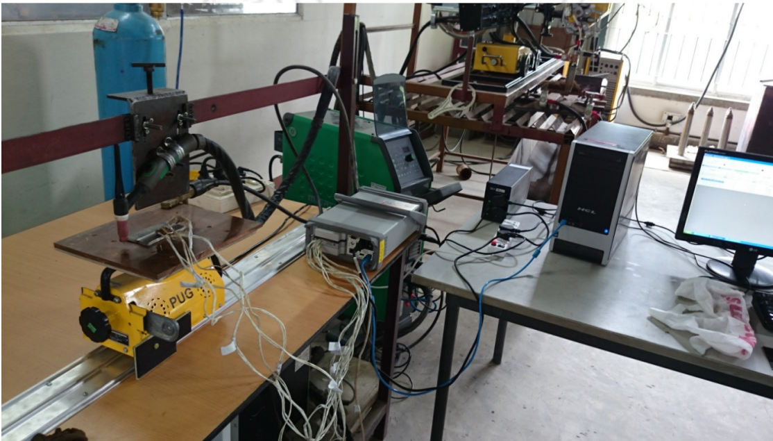
Figure 4.34: In-house developed GTA welding experimental setup along with thermocouples.
