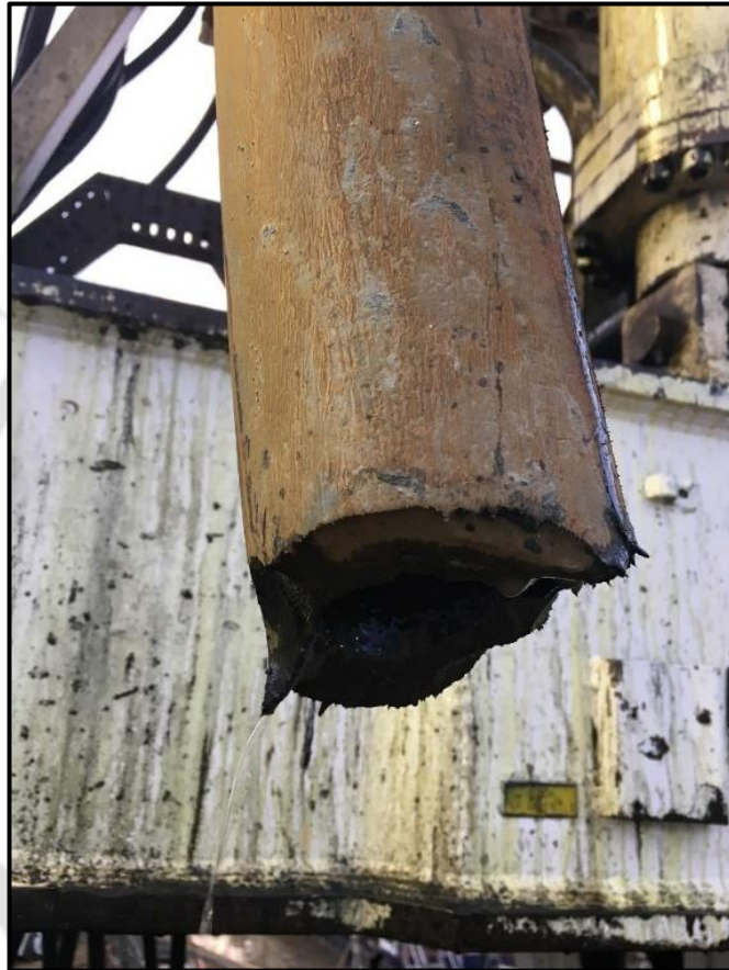
Fig. 1-10. Picture depicting the broken section of the drill string
