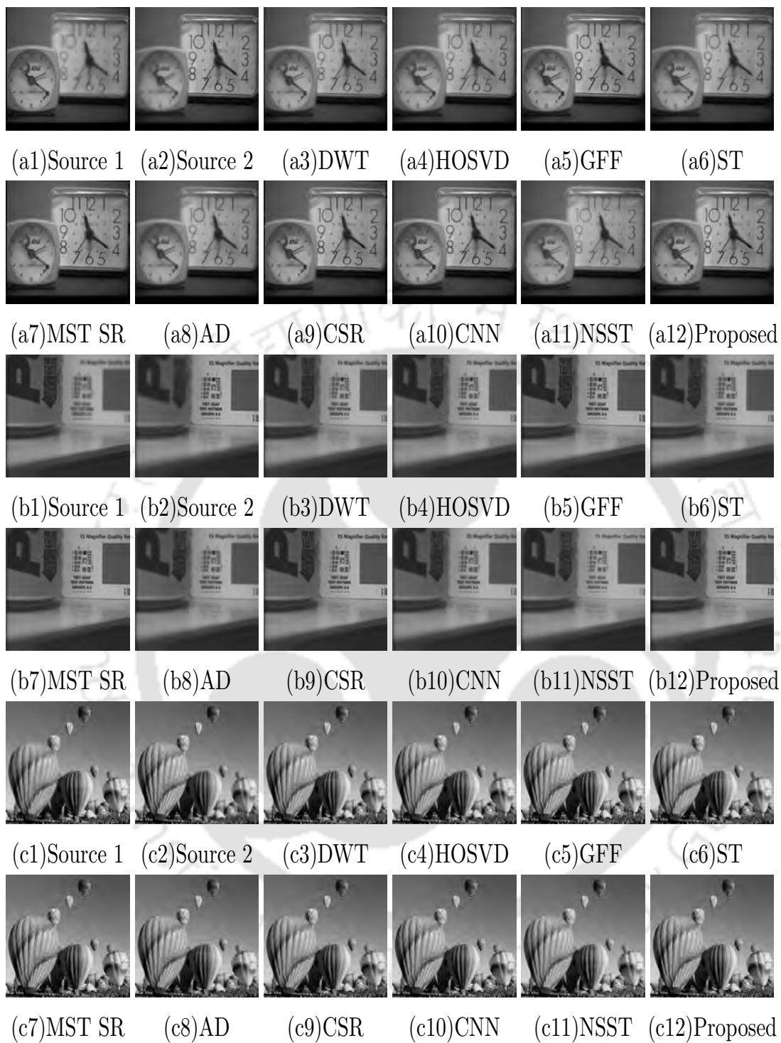
FIGURE 3.8: Multi-focus source and the corresponding fused images obtained by using different image fusion methods.
