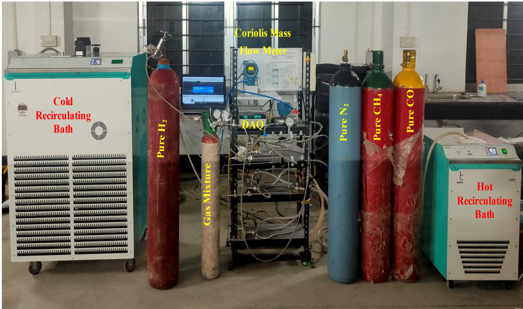
Fig. 4.4 Pictorial view of the 3-stage MHPS
