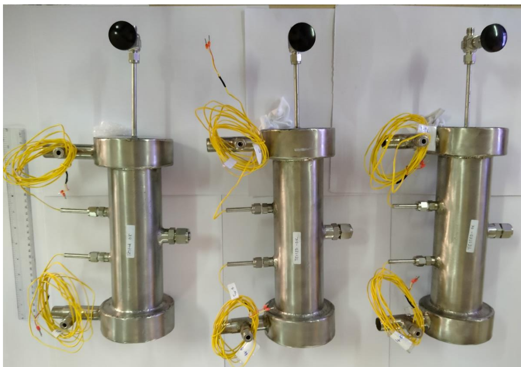
Fig. 3.9 Pictorial view of reactors filled with 1.2 kg of \text{La}_{0.9}\text{Ce}_{0.1}\text{Ni}_5 , \text{LaNi}_5 and \text{LaNi}_{4.7}\text{Al}_{0.3}
