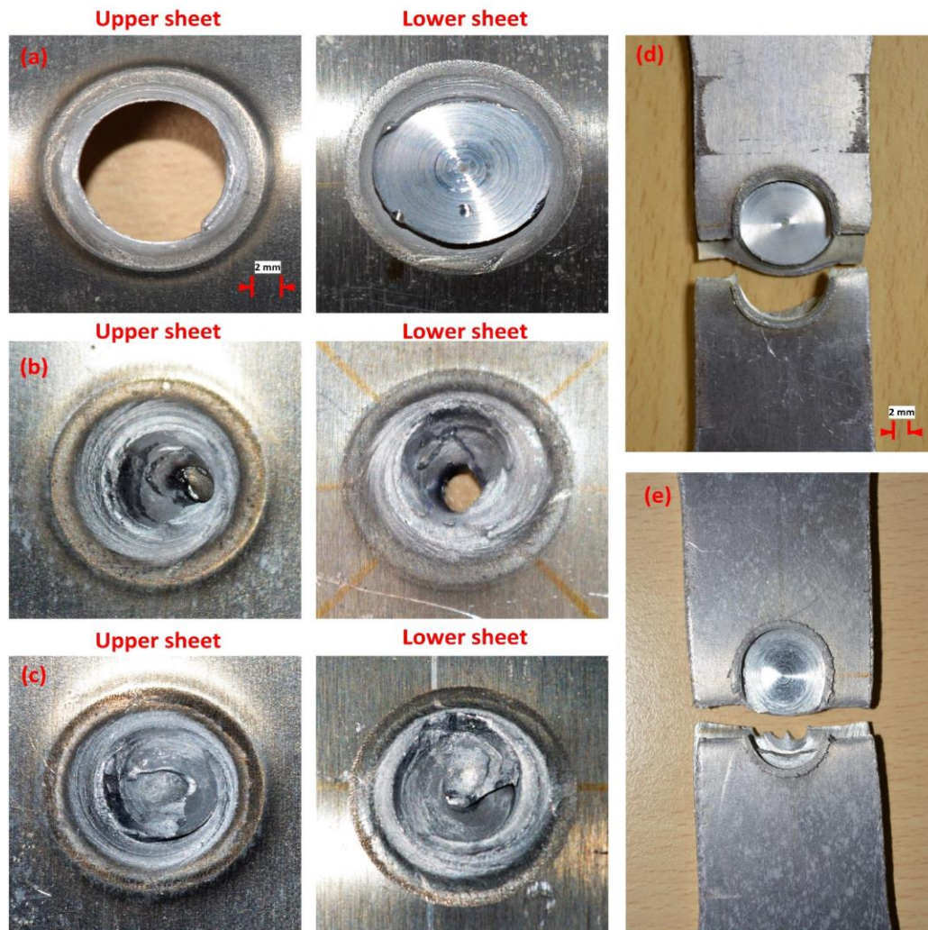
Figure 6.9. Modes of failure. (a) Tear-off, (b) Combine pin pull-out and bond delamination, (c) Combined pin shear and bond delamination, (d) Base metal fracture and (e) Stir spot fracture
