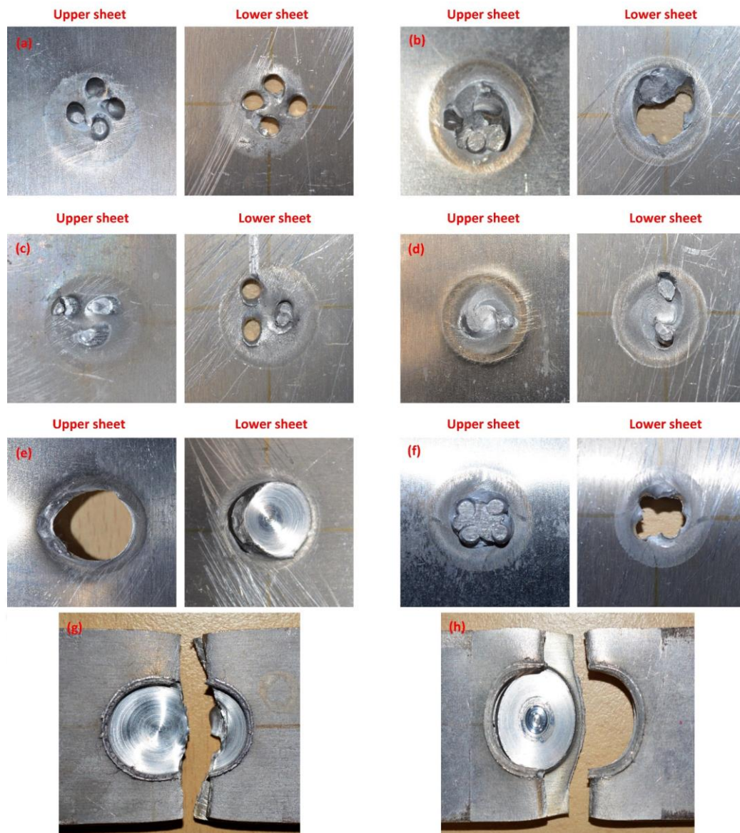
Figure 7.8. Modes of failure. (a) Pin pull-out, (b) Combined pin pull-out and bond delamination, (c) Pin shear, (d) Combined pin shear and bond delamination, (e) Tear-off, (f) Combined tear-off and pin pull-out, (g) Stir spot fracture and (h) Base metal fracture
