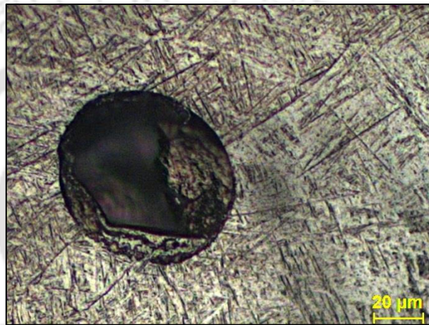
Fig. 5.18 Coalescence of porosity in FZ for samples in Exp. 7
