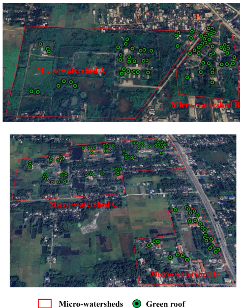
Figure 7.13: Potential location of green roof
