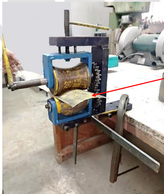
Figure 4.36: Prototype of Shaping tool with gear
