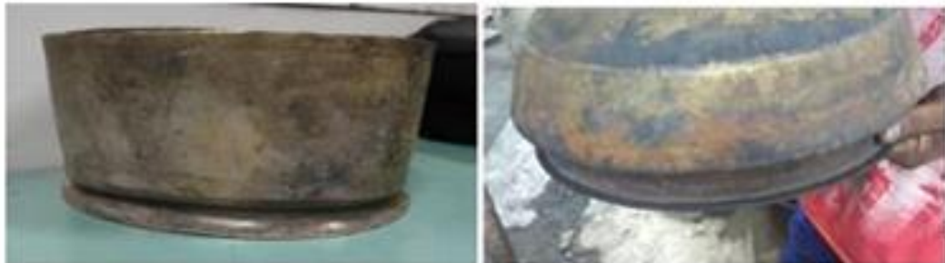
Figure 4.26: Hemming in brass sheet. metal
