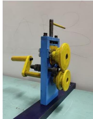
Figure 4.17: Physical model Hemming tool as concept2 view1 Figure 4.18: Physical model Hemming tool view2
