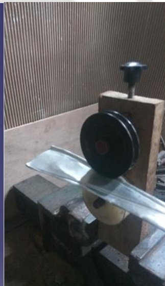
Figure 4.13: Prototype of hemming tool concept 1
