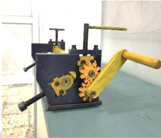
Figure 4.47: Side View of surface bending tool with gear
