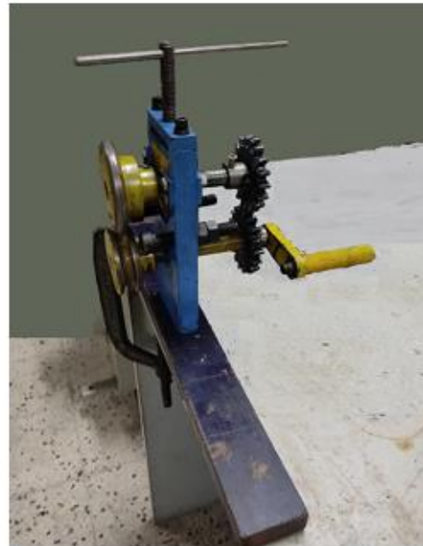
Figure 4.24: CAD model of Hemming with gears Figure 4.25: Prototype of Hemming tool with gears
