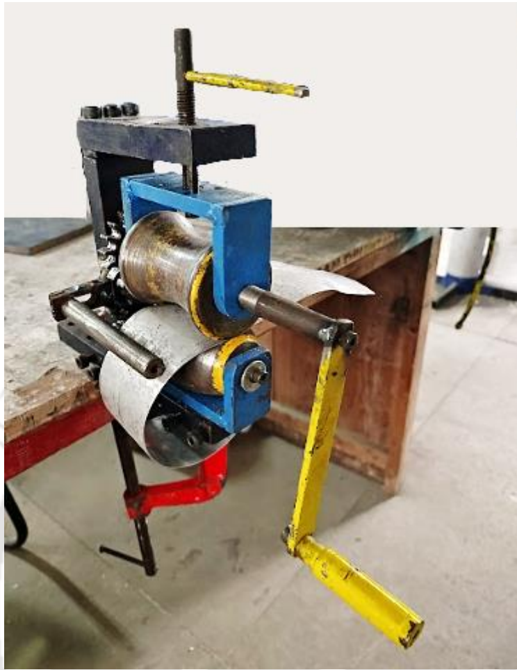
Figure 4.38: Modified shaping tool with gears
