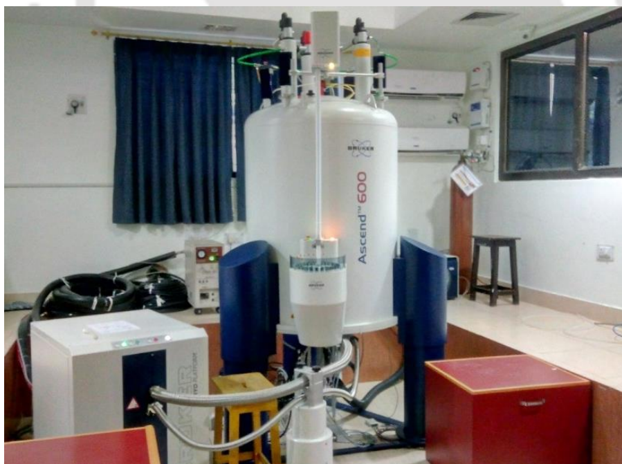
Fig. 2. 7: 600 MHz NMR (Ascend™ 600 Bruker) at central instrumentation facility, IIT Guwahti
