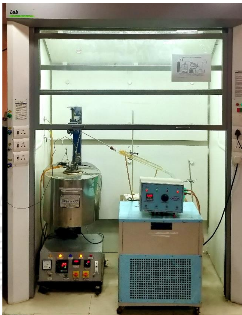
Fig. 2. 5: Semi-batch pyrolysis setup at energy conversion technology laboratory (ECTL) at Department of Chemical Engineering in Indian institute of technology Guwahati, Assam (India)
