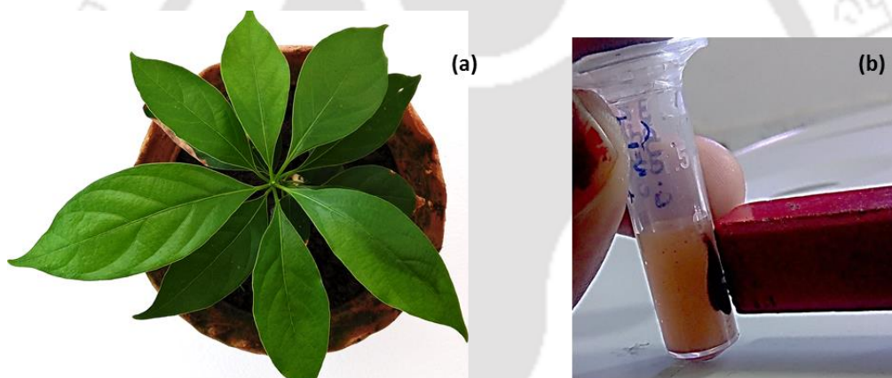
Figure 4.1 Green synthesis of iron oxide nanoparticles using (a) P. bombycina , (b) Magnetic separation of PbFeONPs
