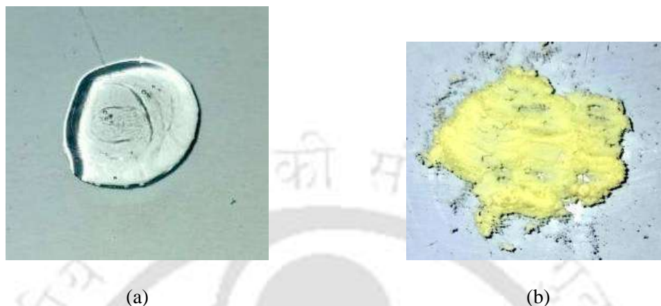
Figure 3.14 Materials used for storage stability analysis: (a) PPA, (b) sulfur
