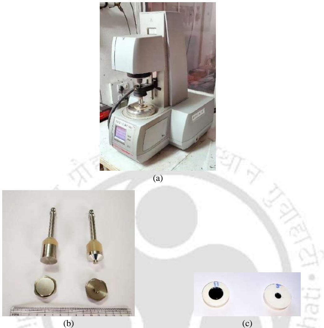
Figure 3.19 (a) DSR instrument used in the study; (b) DSR parallel-plate geometries: 25 mm (left) and 8 mm (right); (c) silicone rubber moulds: for 25 mm sample (left) and for 8 mm sample (right)
