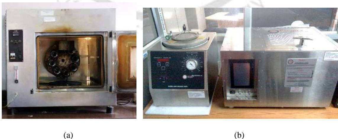
Figure 3.23 (a) RTFO used for short-term ageing; (b) PAV used for long-term ageing
