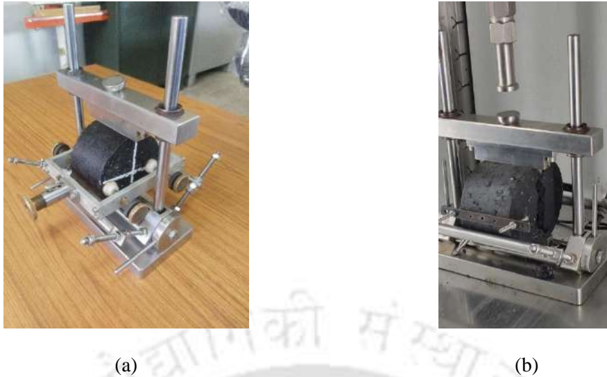
Figure 3.44 (a) Test assembly for ITFT, (b) fractured specimen in ITFT
