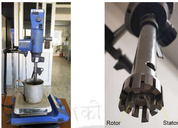
Figure 3.5 High shear mixer (left) and rotor-stator assembly of the high shear mixer (right)
