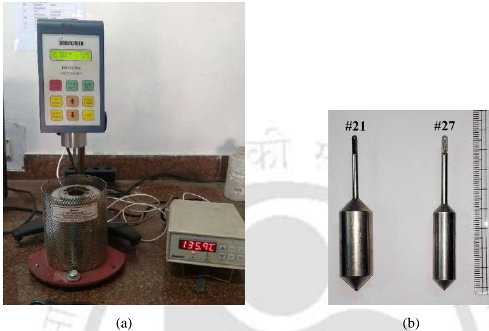
Figure 3.32 (a) Brookfield rotational viscometer, (b) spindles used in rotational viscometry
