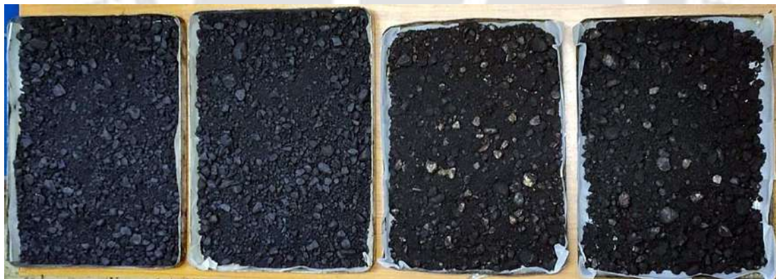
Figure 7.10 Photographs of TPC-10 mixes prepared using mixing temperatures derived from (left to right): EQ, HSV, SSF, and PA methods
