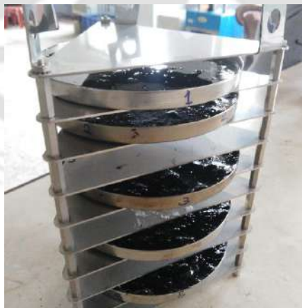
Figure 3.29 Binder samples in PAV pans after undergoing PAV ageing and before vacuum degassing
