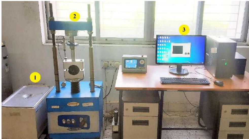
Figure 3.37 Digital Marshall testing system: ① water bath, ② test jig with loading frame, ③ personal computer connected to loading frame
