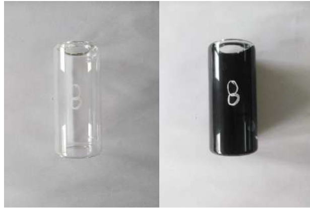
Figure 3.28 RTFO glass bottle before (left) and after the test (right)
