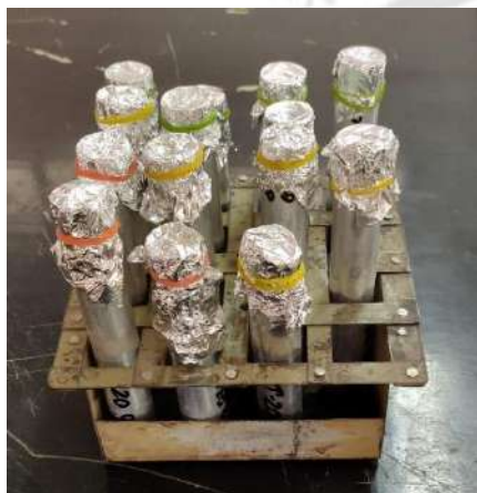
Figure 3.15 Aluminium tubes used in storage stability tests
