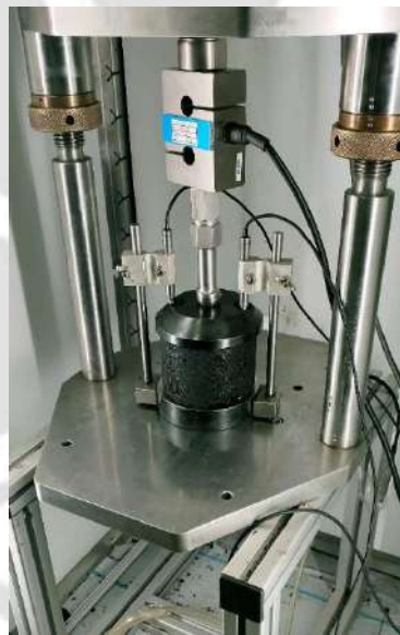
Figure 3.39 Test assembly for static and dynamic creep tests
