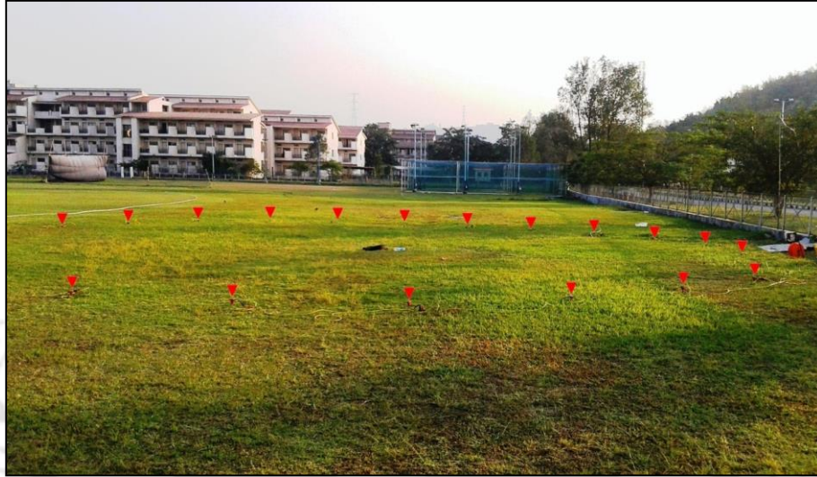
Fig. 9.12 Pictorial view of the circular array used for passive remote survey at Site 1
