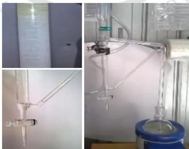
Fig. 2.4: Hydro distillation process using Clevenger apparatus.
