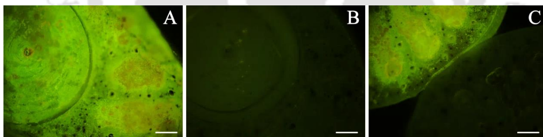
Figure 3.5 Fluorescence microscopic photograph of transverse section of (A) banana pith treated with L 1 , (B) banana pith treated with EDTA first followed by L 1 , (C) banana pith treated with L 1 and banana pith treated with EDTA first followed by L 1 attached together. Scale bar for the images is 200 \mu\text{m} .
