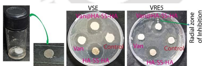
Figure 4.10 Plate images to reveal the antimicrobial efficacy of the Van, Van@HA-SS-HA, and HA-SS-HA against VSE and VRE by zone inhibition method.
