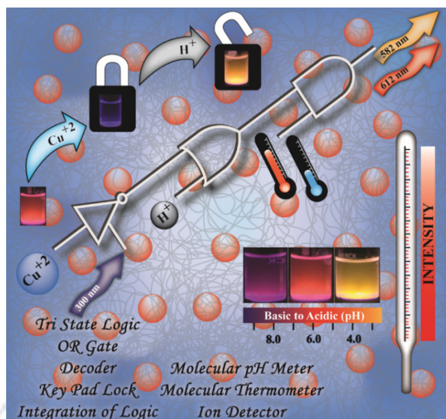
Figure 3.1. Schematic representation of the luminescent atomic cluster-based logically operative molecular devices. The scheme explains the principle of operation of various photonic molecular devices based on luminescent Au NCs in a single liquid system. Boolean logic operations such as tri-state logic, OR gate, decoder, keypad lock and integration of logic to higher levels are achieved. Further its responsive characteristics represent molecular pH meter, thermometer and ion detector.
