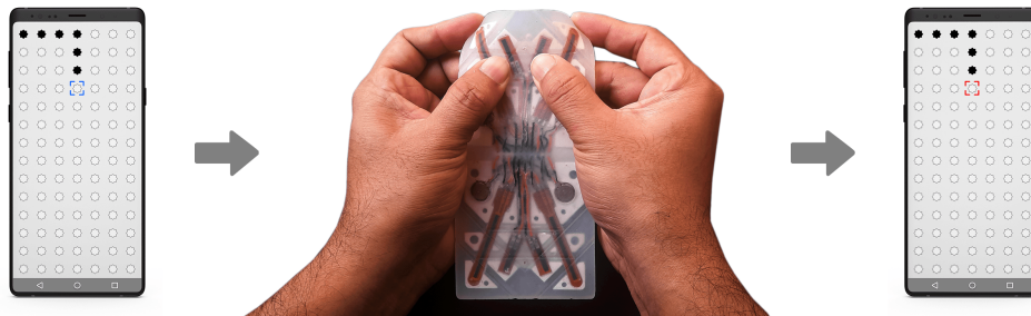
Figure 5.20: A user is performing the Top-corners Bend-upward Small-size gesture combined with On-Crossing a Threshold (or threshold-based) gesture completion strategy to insert a peg. Here, the peg can not be inserted as the current hole in FOCUS is already filled. A warning audio description is provided to the user. (Coloured Figure)
