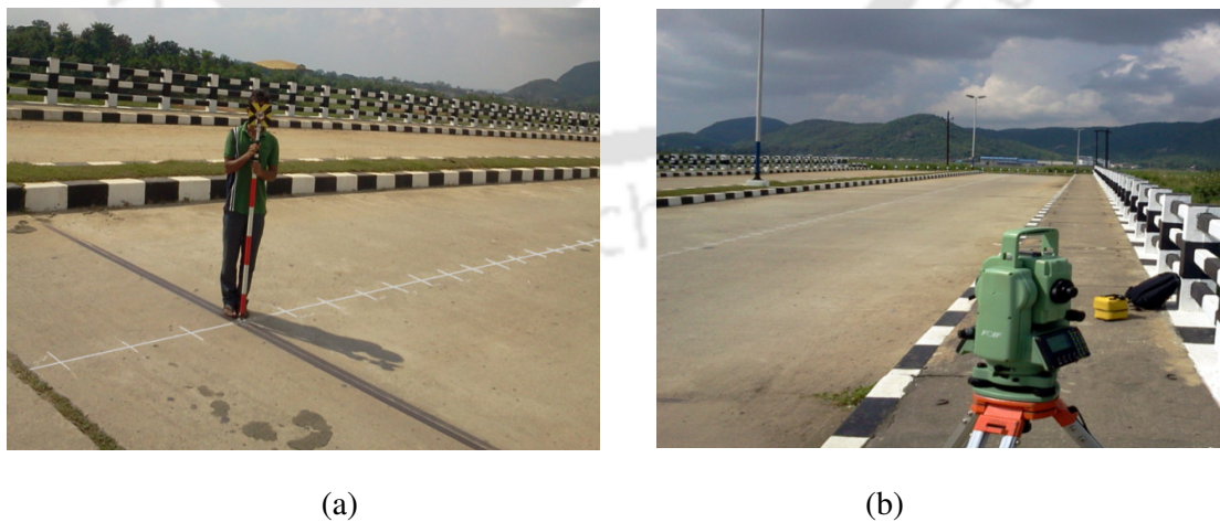
Fig. 5.7 Measurement of bridge deck surface profile (a) Prism with pole placed over the points along the alignment (b) FOIF OTS635 Total Station
