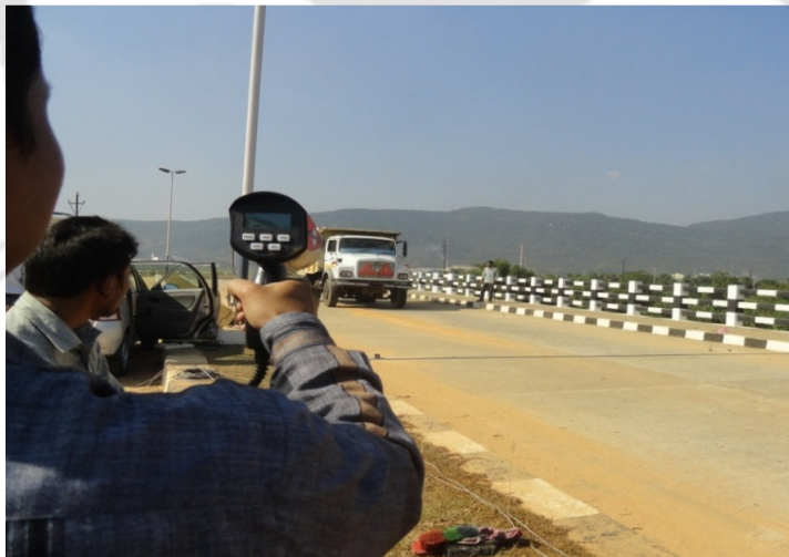
Fig. 5.12 Truck speed measurement using radar gun
