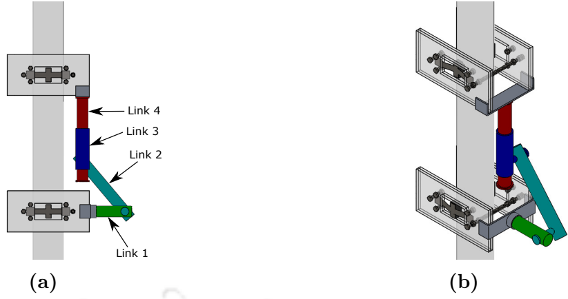
Figure 3.4: (a) Front view and (b) Isometric view of RRRP climbing mechanism for straight vertical climbing
